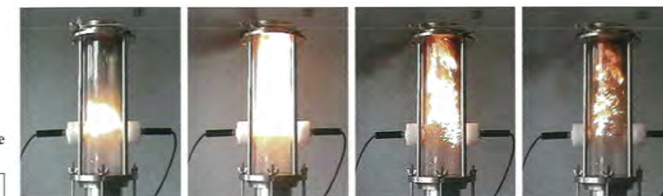
Lower explosive limit measurement
